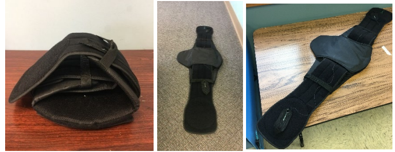
Figure 2. Position of brace for calibration and to test against self-detection, face down on carpet and table, respectively
