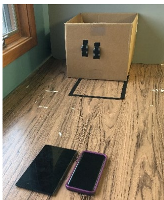
Figure 5. Android devices set 1m from iLink sensors for syncing
