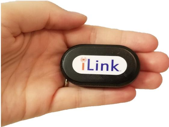
Bluetooth module can be added to any brace
